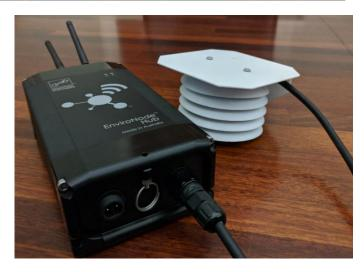
The EnviroNode-PM communicates with the EnviroNode Hub over UART. The EnviroNode Hub manages the sensor to save power and maximise the sensor's operating lifetime.
